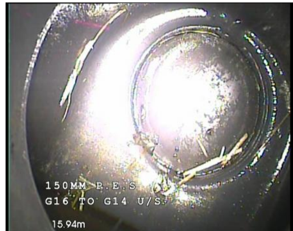
Photo: 17_17_229_A.jpg, 00:02:21 16m, Finish node type, gully reference number: G14 Remarks: TRAPPED GULLY 14
